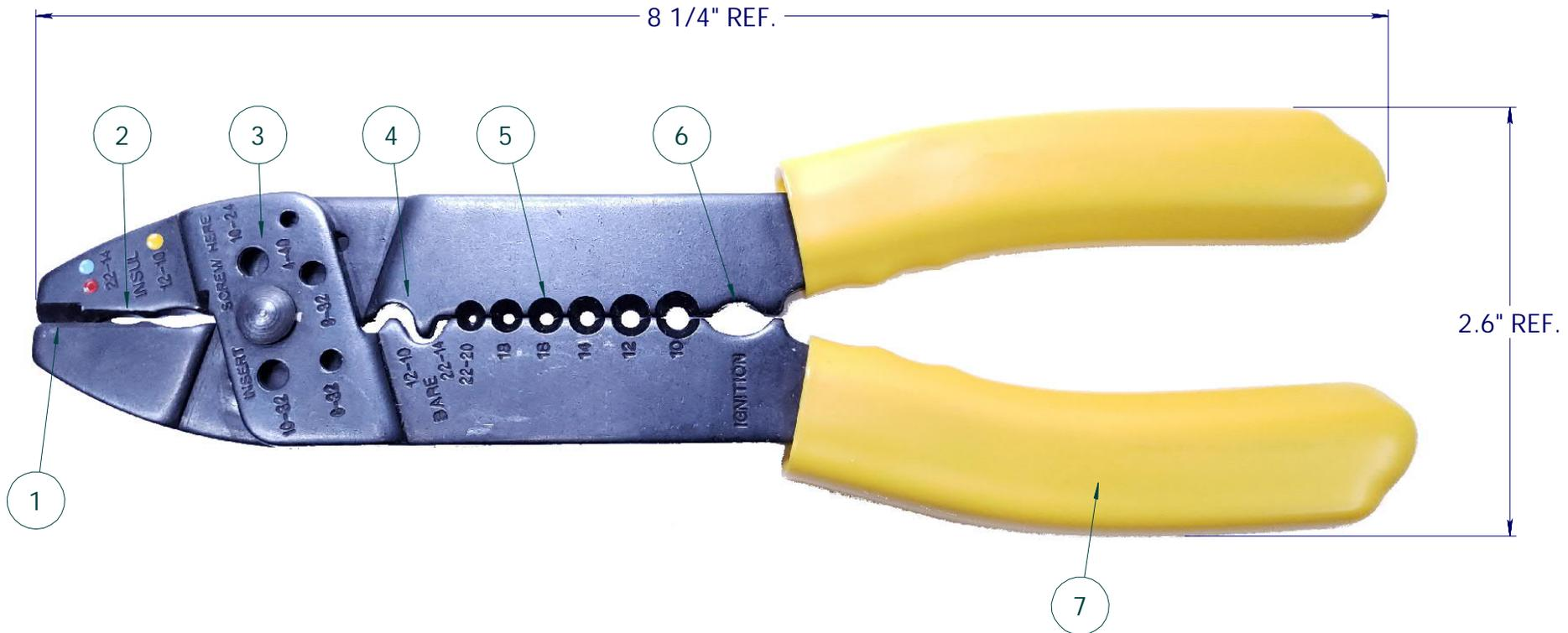
A COMPACT, HIGH-QUALITY TOOL DESIGNED TO HANDLE THE SIX MOST COMMON ELECTRICAL WIRING FUNCTIONS. MADE OF .125" HEAT-TREATED CARBON STEEL FOR MAXIMUM DURABILITY. IT HANDLES A VARIETY OF TERMINAL AND CONNECTOR STYLES, INSULATED AND NON-INSULATED, OVER A RANGE OF 22-10 AWG.
